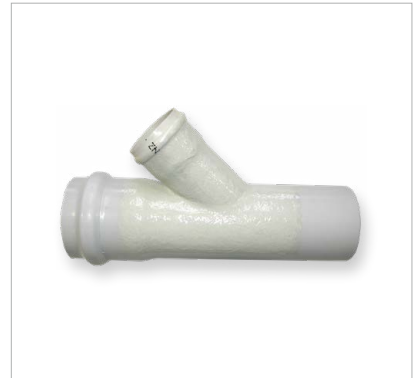
FIG. 12 45° Sewer junction SN16 collar/spigot 150 x 100 x 45°
