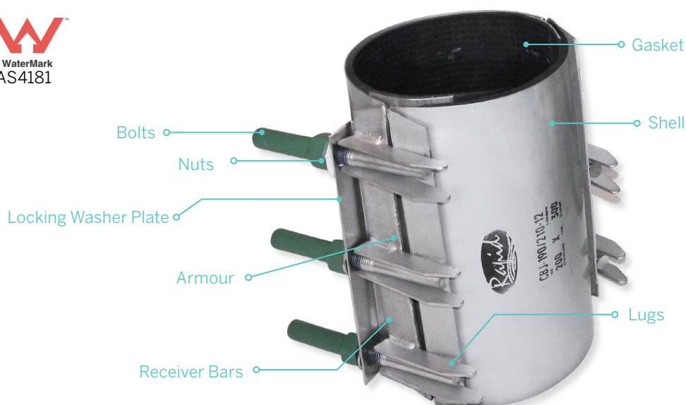
FIG. 1 200mm Rapid Repair Clamp
