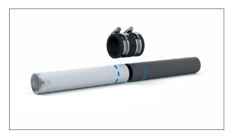
1. Mark both pipes, from the end to be connected, half the width of the coupling, less the required joint gap, which is usually  $10\,\mathrm{mm}$
